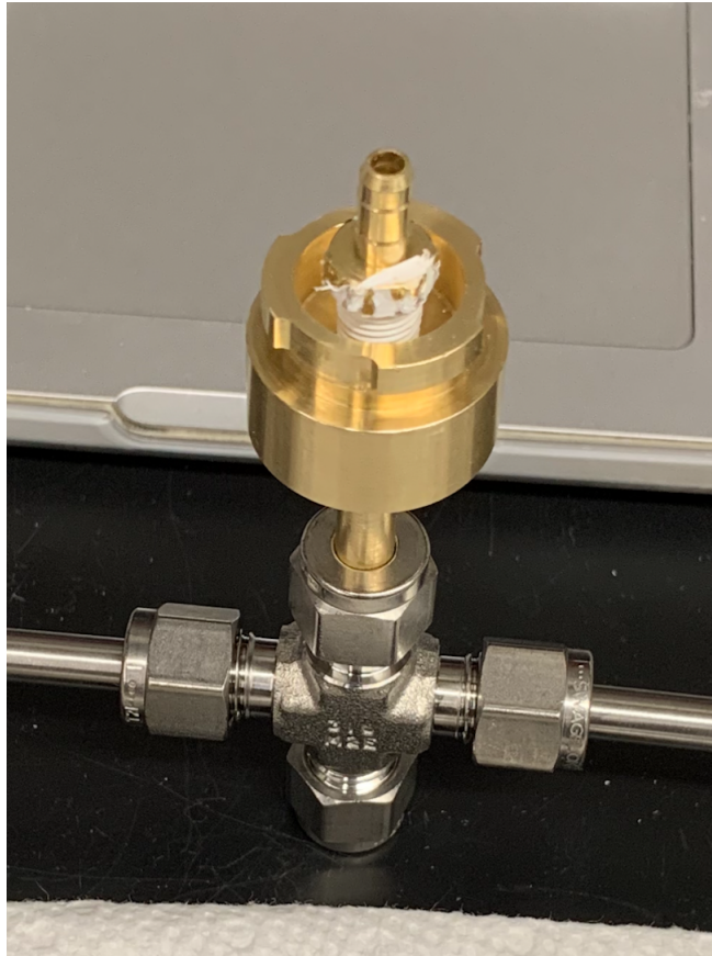
Figure 18: Machined brass connection piece with the barbed tube fitting.
